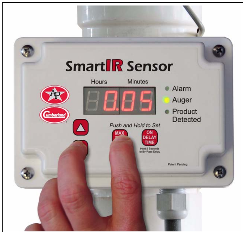
Figure 6C Adjusting the Maximum Run Time
