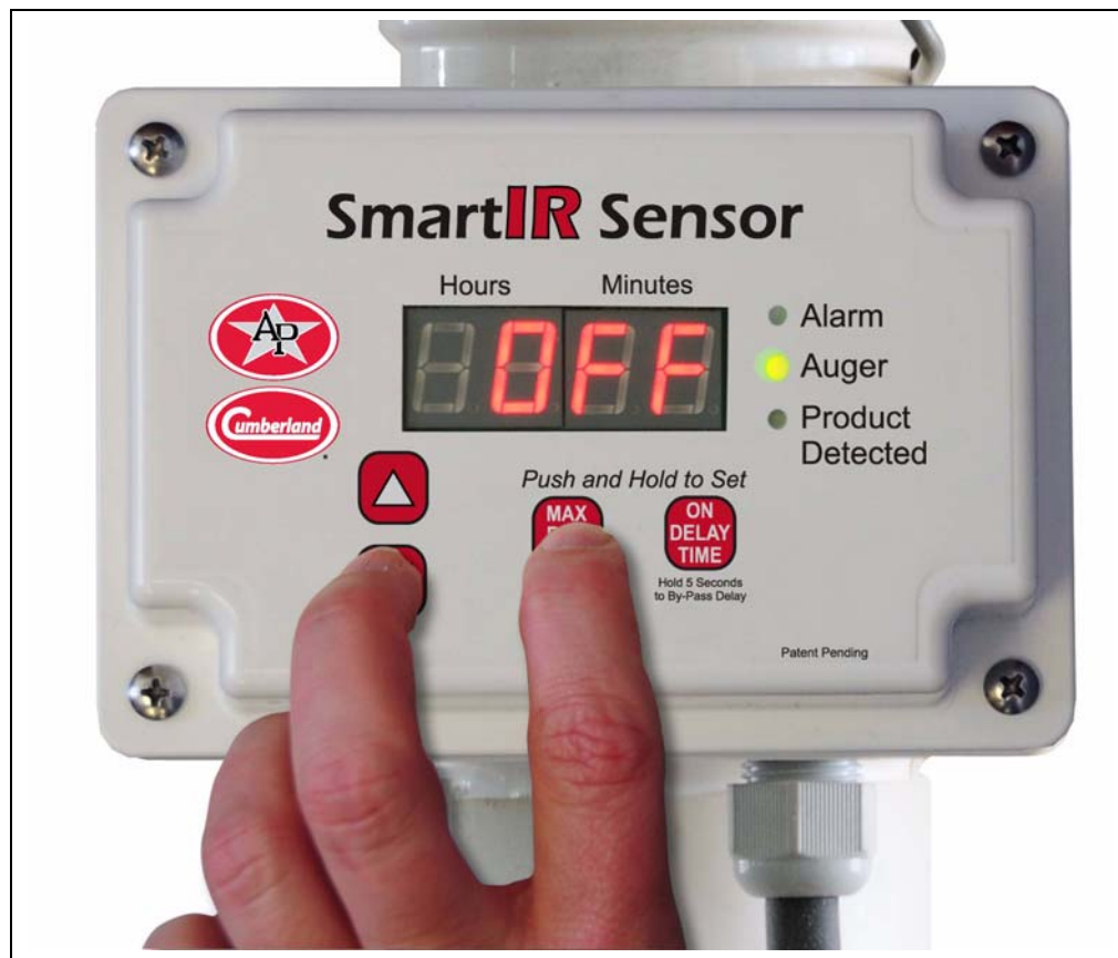
Figure 6D Disabling the Maximum Run Time Feature (Not Recommended)
