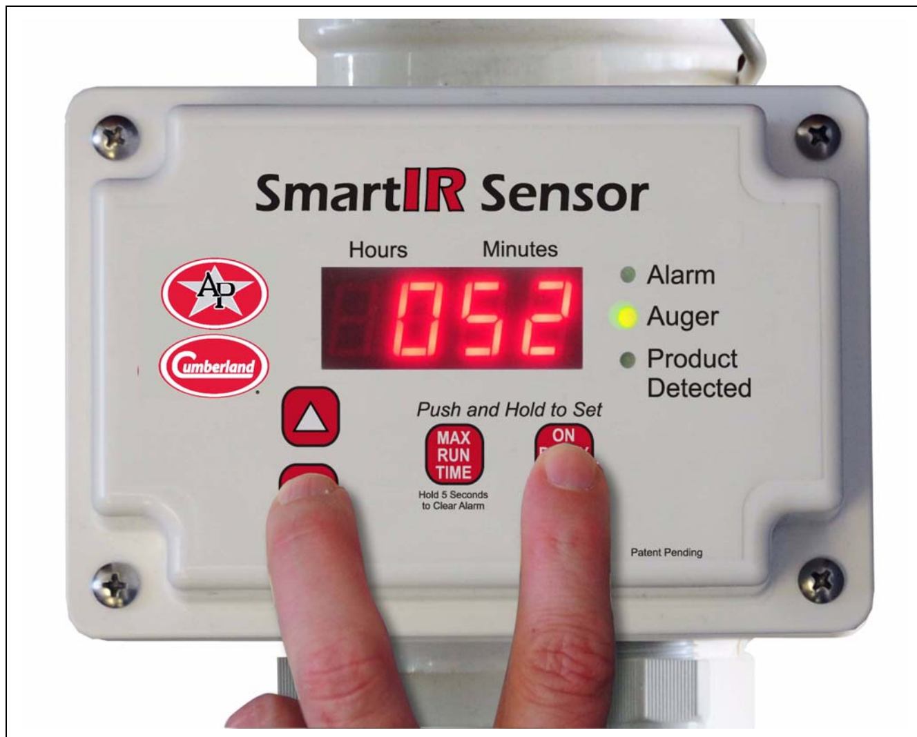
Figure 5B Adjusting the Delay Time
