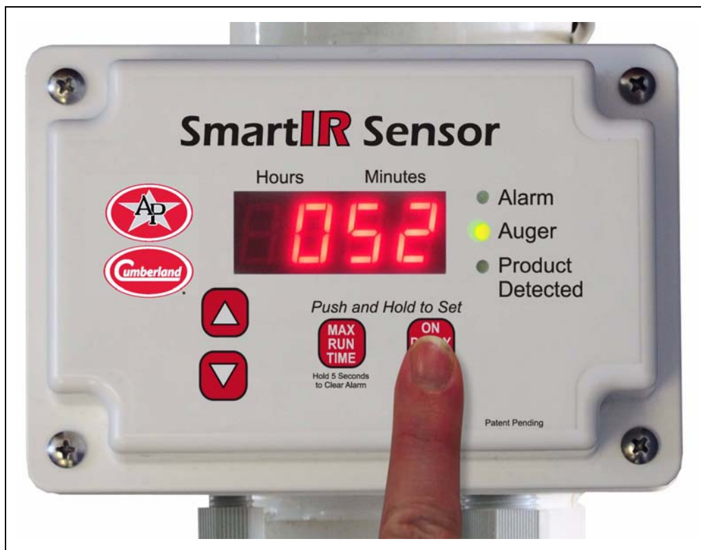
Figure 5A Checking Delay Time
